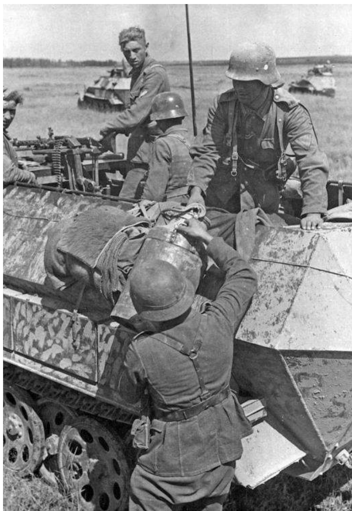
This 251/1 Ausf C belongs to a heavy machinegun squad as evidenced by the sustained-fire heavy MG mount. The vehicle is painted dark grey with mud applied as camouflage. The heavy machinegun section was a support weapon tasked to provide concentrated fire on decisive or threatening positions. At close ranges, it could use a standard MG mount and function as a normal 251/1.
