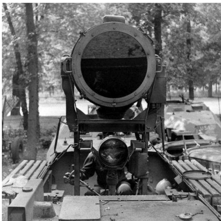
Above: A front view of the searchlight. The operator's sight is visible just below the light. Also visible in front of the light is the generator. Note the walkways on either side of the hull to service the light.
