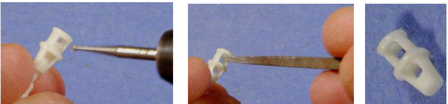
The muzzle brake was plugged with excess resin. A quick touch with a round cutting disk in my Dremel cleaned most of this out. A square needle file took care of any remaining. The result was a one-piece hollow muzzle brake.
