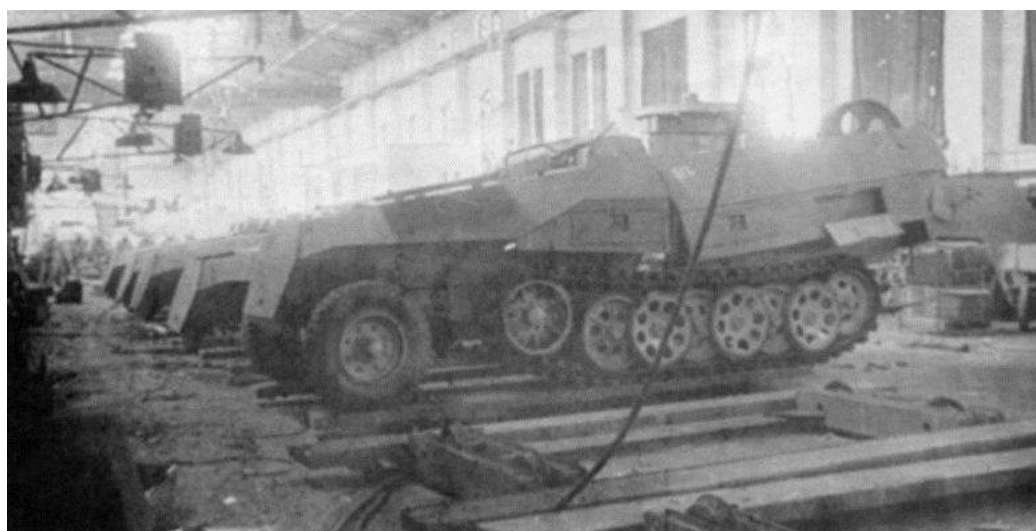
Above: This photo of 251 AusfDs on the production line clearly shows the two part hull. The front and rear portions were joined together directly behind the driver and co-driver's seat.
