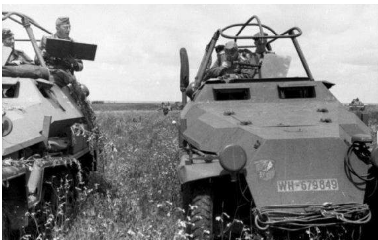
Left: Two Ausf Cs, possibly 251/3s, but more likely (based on the frame antenna) 251/6s. The vehicle on the right is also fitted with a Kurbelmast on the right rear. Right: Vehicles served as long as they were above. This is an older 251/6 Ausf B still in service in 1944. Note the extra side stowage locker on the fender.
