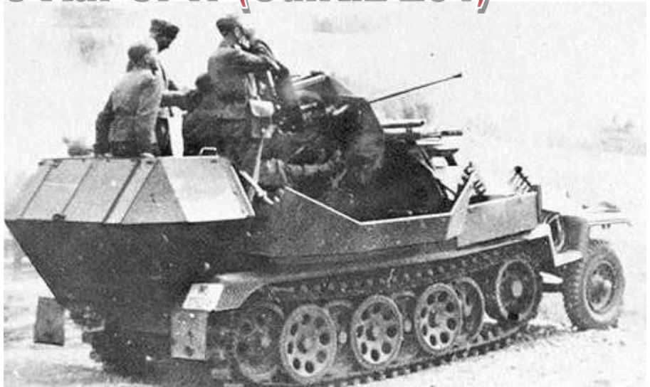
The Luftwaffe's 2cm Flak 38 Auf SPW with sides folded down to engage ground targets. Only a handful of these vehicles were made. Although never given the 251/17 designation (the vehicle was built in 1942 and the 251/17 designation was not used until late 1944), I have included the vehicle here as most references (and, indeed, model companies) list it as a 251/17 Ausf C.
