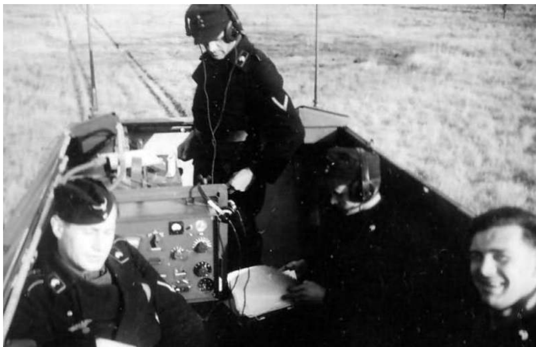
A view showing the radios and rack mounted in place of the right rear bench seat. Different radios/communications equipment were carried by different 251/3s based on mission and sub-variant as follows:
