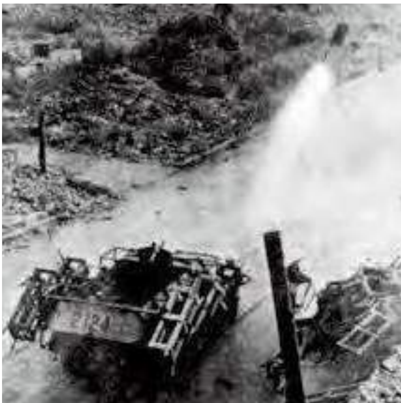
Above: Launching the rockets. Note the pile of used firing crates discarded by the vehicle. Below: A good view of the Wurfrahmen 40 fitting to a 251/1 Ausf C. The angled bars on the inside edges of each front fender were used by the driver to "aim" the vehicle toward the target. Elevation of the rockets was adjusted on the platforms themselves. This crude aiming was all that was necessary—the inherent inaccuracy of the rockets rendered any finer aiming useless.
