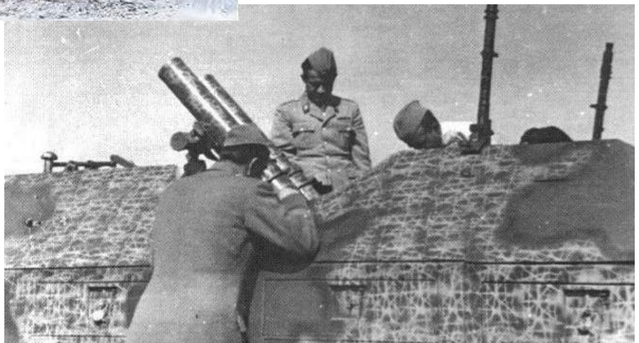
Right: This Ausf D was captured and used by Yugoslavian partisans. The vehicle is fitted with twin 120mm mortars. Note how a semi-circle has been cut from each side of the halftrack to allow the mortars to fully rotate and depress in all directions. Note the very intricate and unusual camouflage pattern on the vehicle—even carried onto the gun tubes. There also appear to be expedient mountings for 2 MG 34s—one mount on each side at the front of the fighting compartment.
