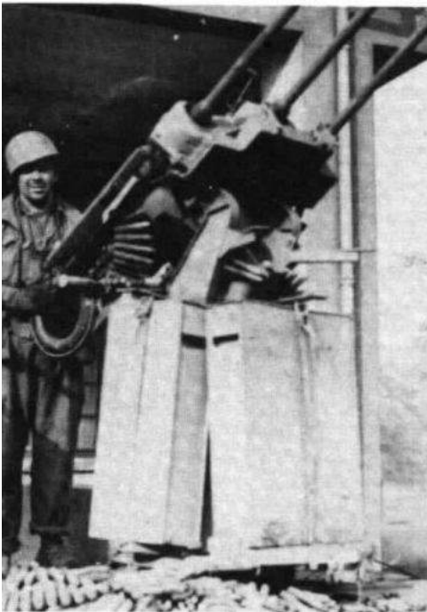
Above: The Drilling weapon system. The three large boxes mounted on the pedestal are the ammunition feed bins. Ejected shells were feed into the central pedestal.
