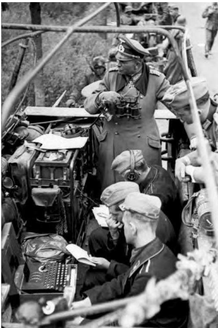
Above: The radio rack taking the place of the rear right seat.
