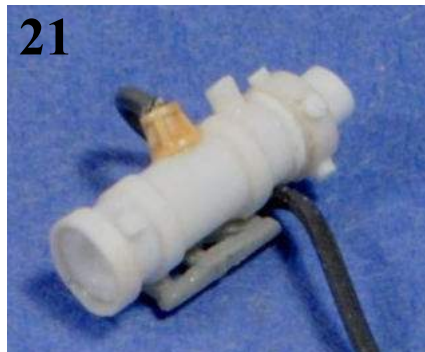
20-21) The scope for the driver was made by first making a basic form from plastic rod detailed with plastic strip. A base was fashioned from an old piece in the scrap box (bottom left). The scope was then detailed with slices and lengths of plastic rod. The cable attachment is part of a spare Tamiya antenna mount, and the cable itself is more of the rubber string (bottom right).
