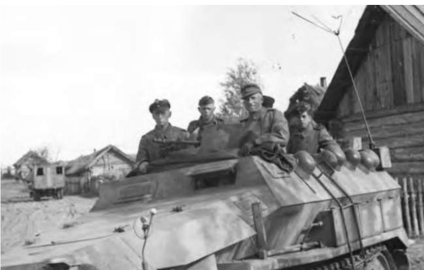
Left: This 251/3 carries a star antenna on the rear of the right side of the hull. There does not seem to have been a standard location of the various antenna. Photos show a variety of combinations and locations. One photo shows the Kurblemast being mounted inside the fighting compartment behind the driver's seat!
