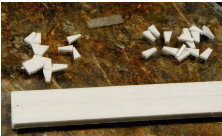
The magazine racks were made from a thick piece of plastic bar stock and wedges cut from a 4mm x 1mm plastic strip. I cut wedges as the magazines are curved and the ends projecting from the rack would not be completely vertical. The wedges, 30 per rack were glued in place and the racks glued into the vehicle hull. Note that the base of the gun mount must be put in place first or it will not fit into the hull. The dead guy is in place only for a test fit.
