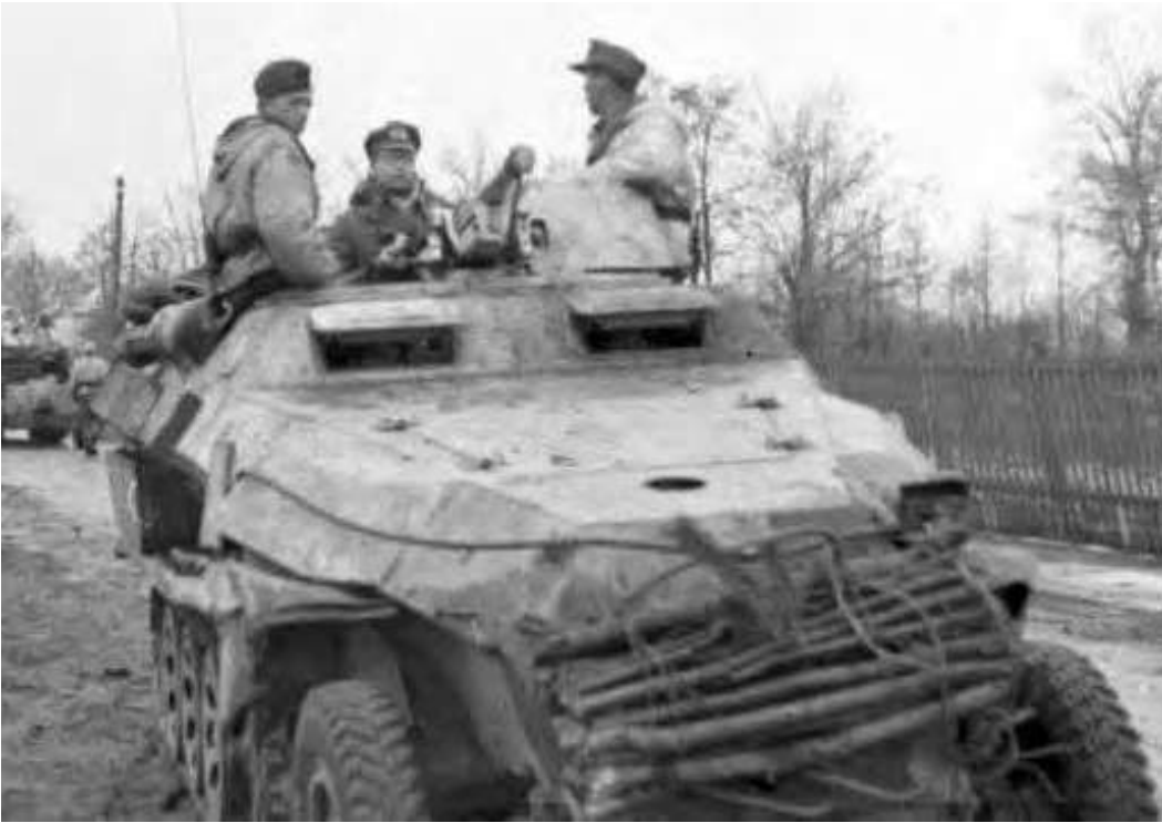
Left: A factory-built 251/10 Ausf C. The bundle of logs on the nose are to assist with un-ditching or negotiating soft ground. This old veteran is battered—note the missing front fenders and radiator cap cover
