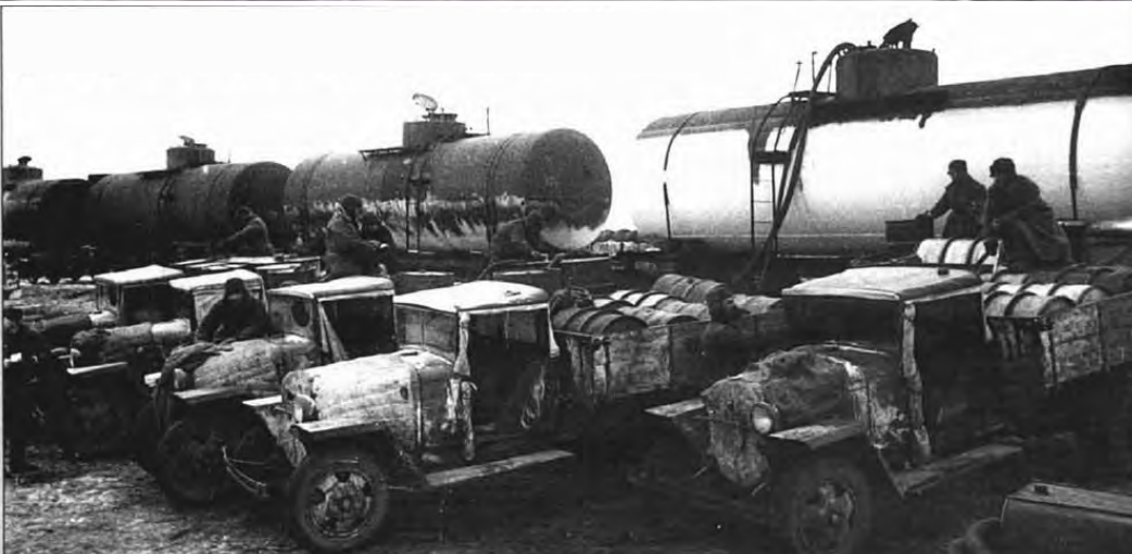
Trucks cross-loading fuel from railcars. The vehicles appear to have worn winter whitewash.
