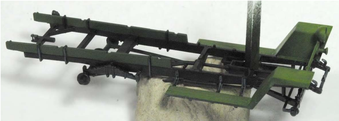
The frame, chassis, and fender assembly to this point. (The plastic rod is a length of styrene glued into the hollow engine to serve as a handle for painting—it will be snipped off flush with the top of the engine before the cab assembly is glued in place).
