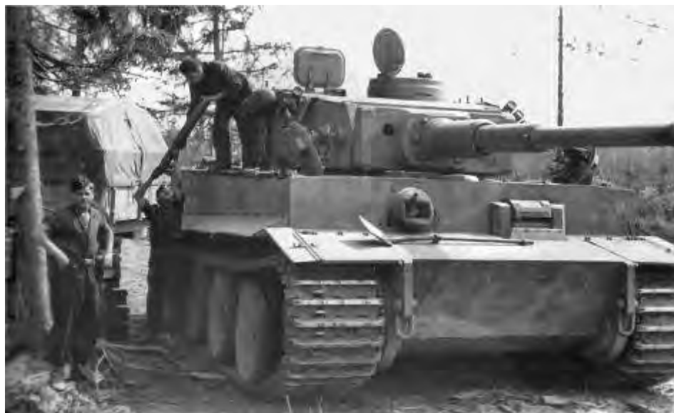
This photo of a tank taking on ammunition gives us a good view of the front of an early-production Tiger. Note the shovel mounted on the glacis, the hinged front mudguards (with hinged side flap), side mudguards with triangular ends, smoke candles on the turret, and S-Mine dischargers on the hull. The photo also gives a clear view of the crew hatches and shows the interleaved wheels. This vehicle also features the loader's periscope and spare track links on the turret fitted beginning in March, 1943.
