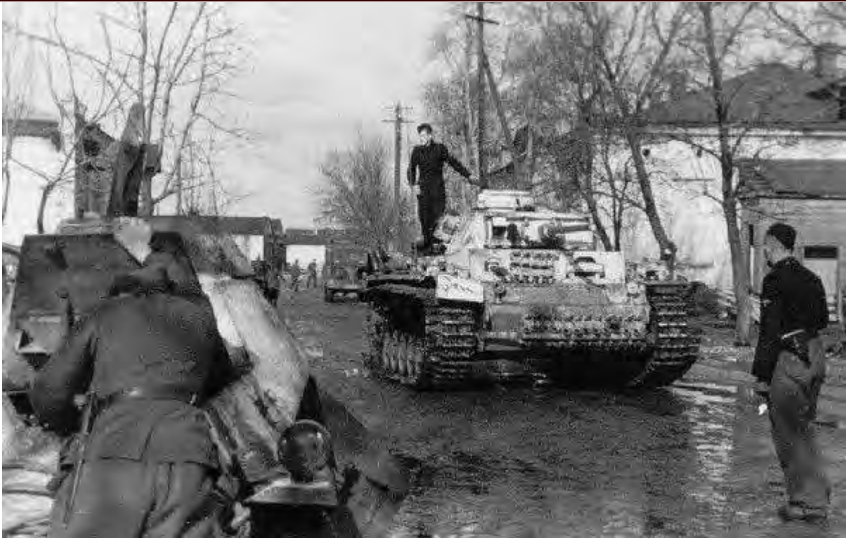
Above: German troops perform maintenance on a captured BA-64. In the road is a Panzer III fitted with wide Winterketten tracks to increase flotation/mobility on soft ground.
